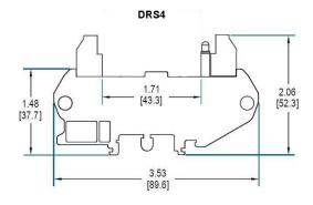
$$\label{eq:total_control_control} \begin{split} & \text{Tolerances:} \pm 0.02 \text{ in / 0.5 m} \\ & \text{All dimensions are in: inches [millimeters]} \end{split}$$
