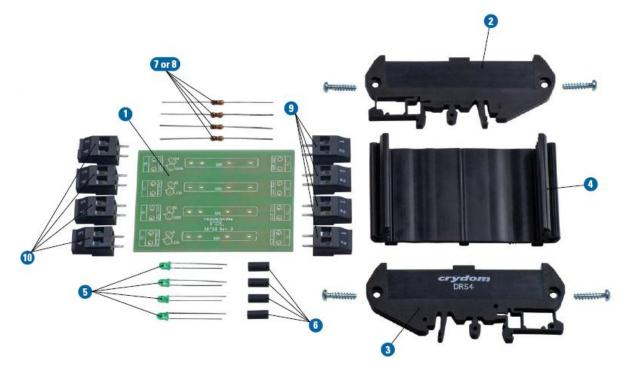
(E) Use 1K  $\Omega$  (brown-black-red) resistor for applications with control voltage range between 3-15 Vdc and 4.7K  $\Omega$  (yellow-violet-red) resistor for applications with control voltage range between 15-32 Vdc. LED status indicator is not required for proper function of the SSR and may be omitted. No resistors are needed when LED is not installed. For AC input SSR control applications LED status indicator and resistor must not be used. SSR(s) purchased separately.
