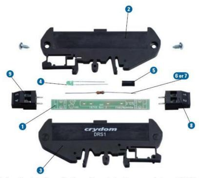
(E) Use 1K  $\Omega$  (brown-black-red) resistor for applications with control voltage range between 3-15 Vdc and 4.7K  $\Omega$  (yellow-violet-red) resistor for applications with control voltage range between 15-32 Vdc. LED status indicator is not required for proper function of the SSR and may be omitted. No resistors are needed when LED is not installed. For AC input SSR control applications LED status indicator and resistor must not be used. SSR(s) purchased separately.
