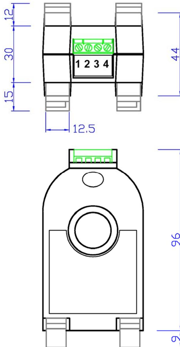
5. Dimensioned Drawing (Including Rail MountClips)
