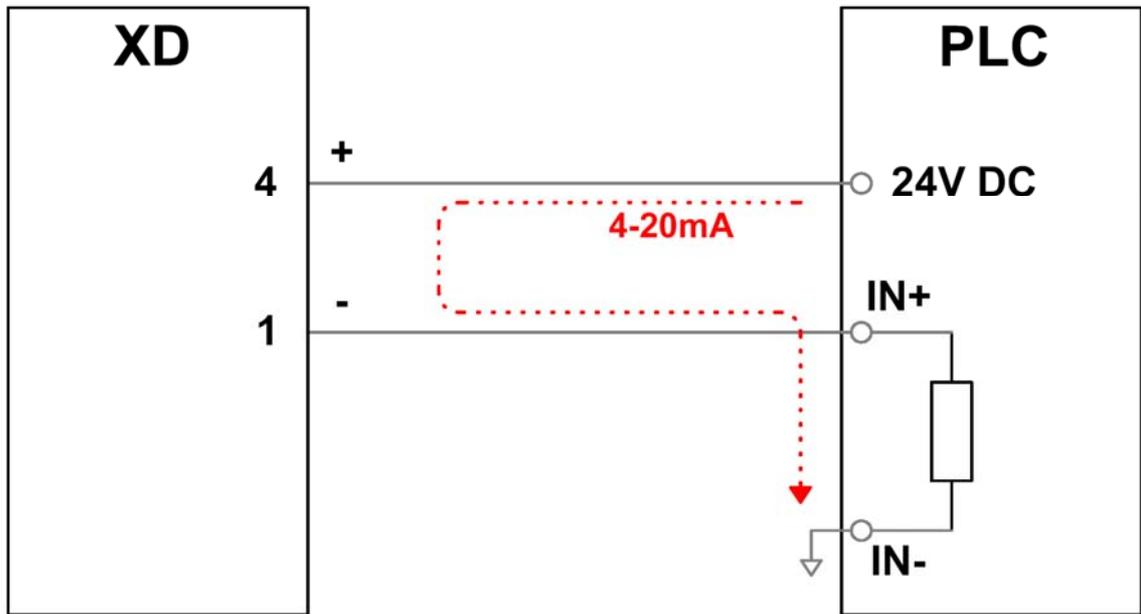
8. Typical 4-20mA Connection Loop Powered
