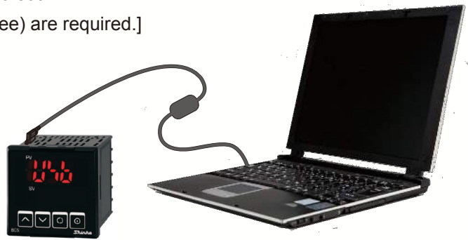
Power to the BCx2 is supplied by PC via USB.
