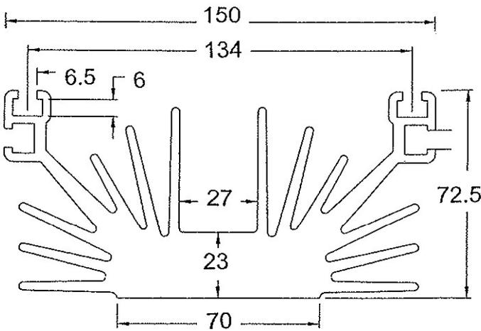
The H8 Heatsink is mostly used for all "Puk" or Capsule devices in double side or single side cooling arrangements. The construction of the heatsink allows the user to attach RC- snubber networks or fuses. To obtain the lowest possible thermal impedance H8 heatsink can also be forced air cooled.
