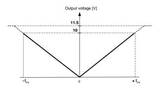
Note: 1) The performance specified in the datasheet is valid within the 0-10 V DC output range only.
