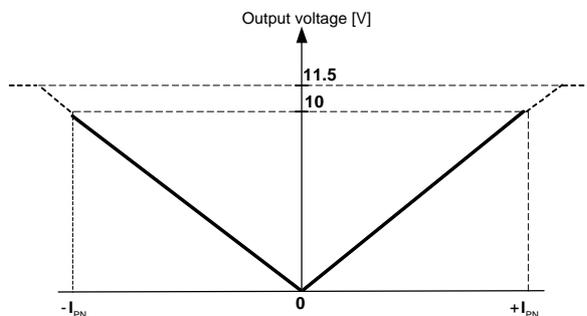
**Note:** <sup>1)</sup> The performance specified in the datasheet is valid within the 0-10 V DC output range only.
