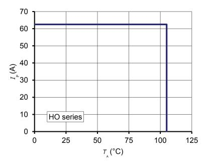
Figure 16:  $I_P$  vs  $T_A$  for HO series
