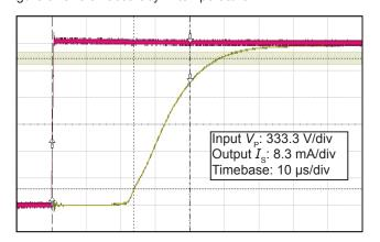
Figure 5: Typical step response (0 to 2000 V)
