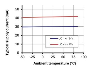
Figure 7: Supply current function of supply voltage
