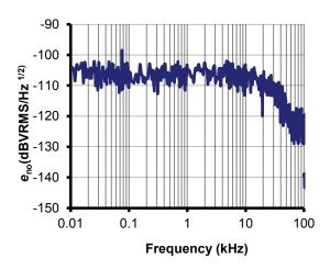
Figure 11: Typical noise voltage density  $e_{\rm no}$  with  $R_{\rm M}$  = 50  $\Omega$
