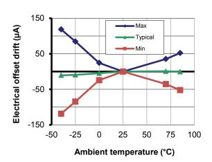
Figure 2: Electrical offset thermal drift
