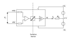
Figure 14: Standard characterization schematics for current output transducers ( $R_{\rm M}$  = 100  $\Omega$  unless otherwise noted)
