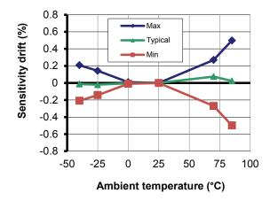
Figure 4: Sensitivity thermal drift
