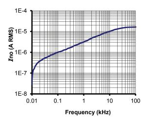
Figure 12: Typical total output RMS noise current with  $R_{\rm M}$  = 50  $\Omega$
