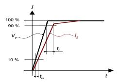
Figure 15: Response time  $t_r$  and reaction time  $t_r$
