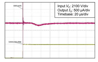
Figure 6: Detail of typical common mode perturbation (4200 V step with 6 kV/ $\mu$ s,  $R_{\rm M}$  = 100  $\Omega$ )
