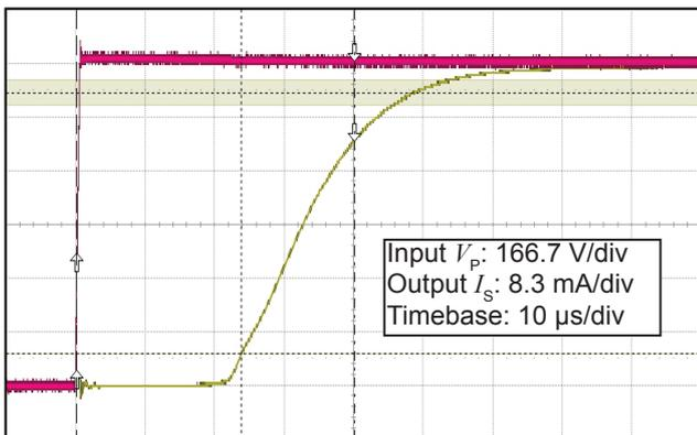
Figure 5: Typical step response (0 to 1000V)
