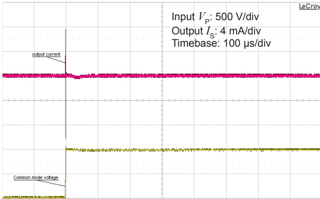
Figure 11: Typical common mode perturbation (1000 V step with 6 kV/μs R_M = 100 \Omega )
