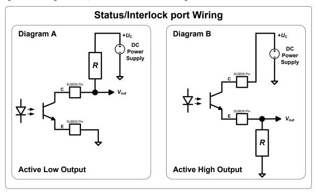
In the Diagram A Active Low Output, the output signal  $V_{\rm out}$  switches to GND when the corresponding LED is ON. In the Diagram B Active High Output, the output signal  $V_{\rm out}$  switches to  $+U_{\rm C}$  when the corresponding LED is ON. When the output signal  $V_{\rm out}$  is switched to GND, its value is lower than 0.2 V. When the output signal  $V_{\rm out}$  is switched to  $+U_{\rm C}$ , its value is equal to  $+U_{\rm C}$ .
