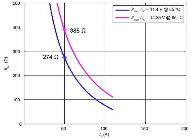
Figure 2: Maximum measuring resistance @ 85 °C in DC
