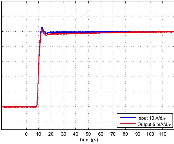
Figure 3: Typical step response (0 to 50 A, 50 A/μs) with  $R_M = 10 \Omega$
