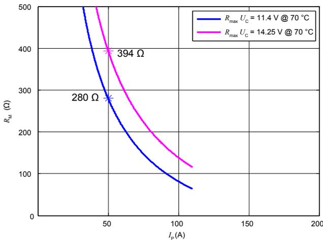
Figure 1: Maximum measuring resistance @ 70 °C in DC
