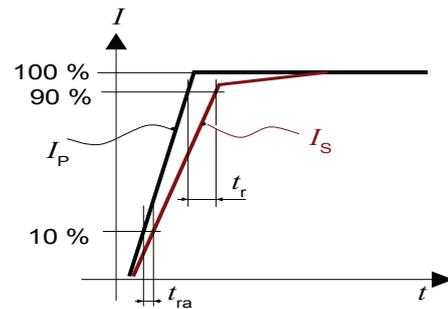
Figure 9: Response time  $t_r$  and reaction time  $t_{ra}$
