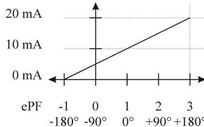
Power angle represents angle between first voltage harmonic and first current harmonic for each individual phase. Total power angle is calculated from total active and reactive power (see equation for Total power angle, chapter *Equations* on page 88). A positive sign shows inductive load, and a negative sign shows capacitive load.
