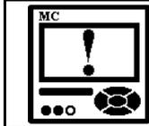
While memory card activity LED is pulsating memory card should not be touched or pulled out of the slot.
