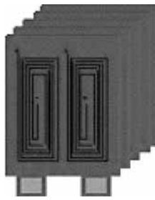
Figure 43: PRiME™ sensor multi-layers printed wiring board
