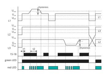
**MVR 56** – RELAY MONITORS PHASE SEQUENCE AND FAILURE (E.G. CONTROL OF CORRECT MO-TOR WINDING ETC.).
