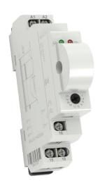
MCR 32 – THE CURRENT TRANSFORMER RELAY, WHICH SENSES THE CURRENT THROUGH THE PASSING WIRE, IS USED TO MONITOR THE HEATING RODS IN THE SWITCHES, THE HEATING CABLES, THE CURRENT FLOW INDICATION, AND THE MONITORING OF SINGLE-PHASE MOTORS.
