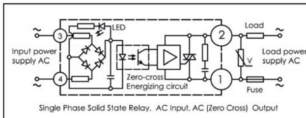
Single Phase Solid State Relay, AC Input, AC (Zero Cross) Output
