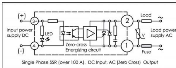
Single Phase SSR (over 100 A), DC Input, AC (Zero Cross) Output
