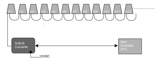
If some I-Link modules are used, they are also connected in the same way through I-Bus short communication cables to another S-Bus converter then to a second Host serial port. Power supply is <u>not</u> yet applied on any of them. Same sequence as for Sentinel must be followed for assigning them unique ID.
