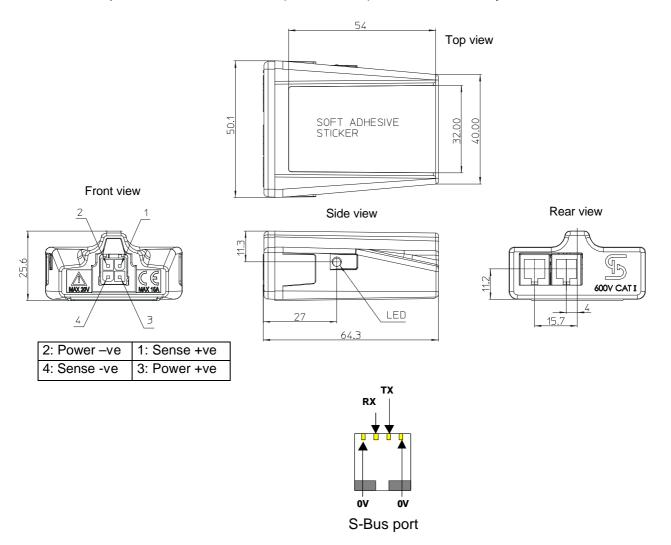
Care must be taken to connect the Sentinel to the positive and negative terminals of the bloc correctly. **Reversal of these leads may damage the Sentinel.**
