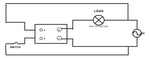
When the switch is open, the light should be off, and with the switch closed, the light should be on. Anything else will indicate a faulty relay.
