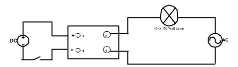
When this is connected, the battery should control when the light is on or off. Applying the 9 volts DC will turn the light on and when you remove the DC voltage, the light bulb should turn-off.
