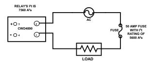
It may happen on some occasions that the "normal" current and voltage ratings required of the fuse push its I<sup>2</sup>t rating close to or beyond the I<sup>2</sup>t rating of the solid state relay. If this is the case, a higher I<sup>2</sup>t rated solid state relay can be selected.
