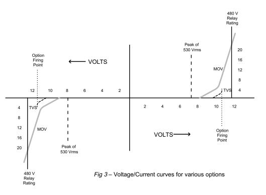
exhibits a very high impedance until its breakover voltage is reached and then breaks down to a low impedance, thus protecting against high voltage transients.
