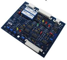
Adjustable Soft-Start: The ISOVLCL-2 includes a potentiometer-adjustable soft-start ramp.
