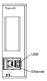
Figure 4-3. Front I/O connectors
