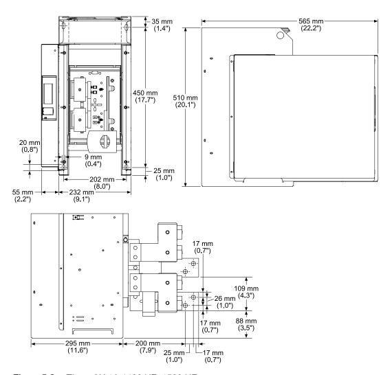
Figure 5-8. Thyro-AX 1A 1400 HF, 1500 HF
