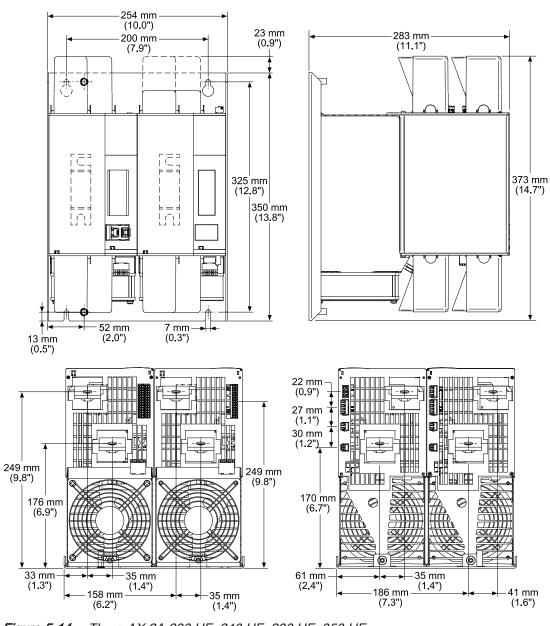
Figure 5-14. Thyro-AX 2A 230 HF, 240 HF, 280 HF, 350 HF
