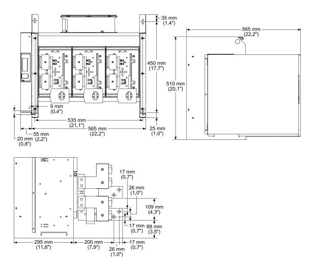
Figure 5-24. Thyro-AX 3A 1400 HF, 1500 HF
