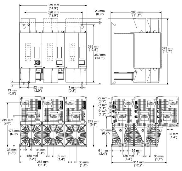
Figure 5-22. Thyro-AX 3A 230 HF, 240 HF, 280 HF, 350 HF
