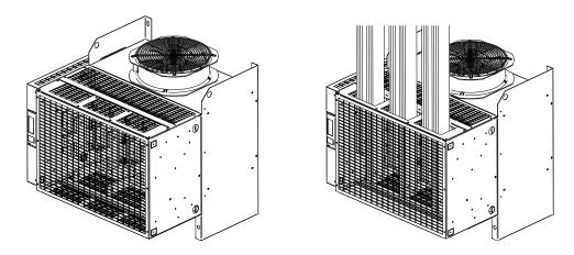
Figure 5-28. IP20 protection, 1000 A through 1500 A
