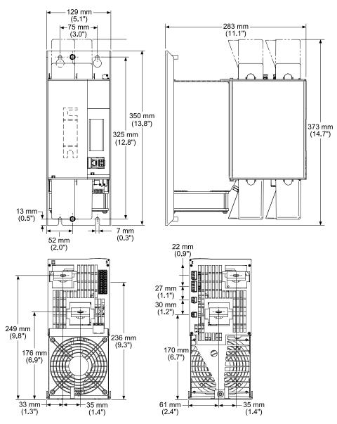
Figure 5-6. Thyro-AX 1A 230 HF, 240 HF, 280 HF, 350 HF
