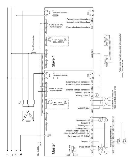
Figure 5-30. 2A power controller connections
