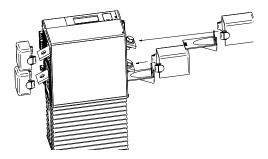
Figure 5-27. IP20 protection, 130 A through 350 A
