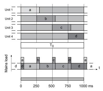
Figure 5-41. Software synchronization
