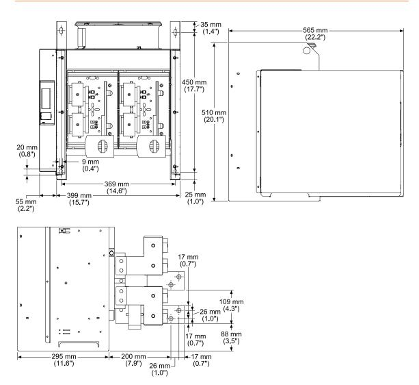
Figure 5-16. Thyro-AX 2A 1400 HF, 1500 HF
