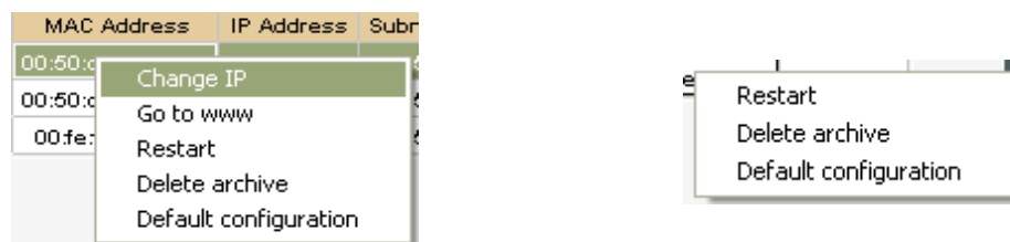
Fig. 19. Menu invoked with a right click (left menu – communication via Modbus TCP, right menu – communication via USB)
