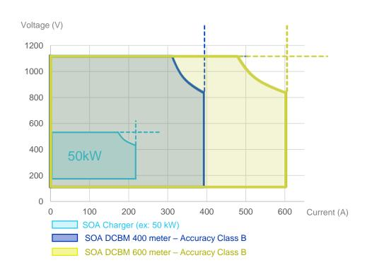
From definition, for PTB, it must be clear that the Shut-Off current of the charging station must be above  $I_{\text{start}}$  of the meter
