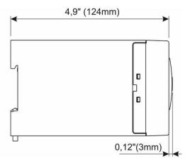
Dimensions for UMT550/560 (ring type terminal block):
