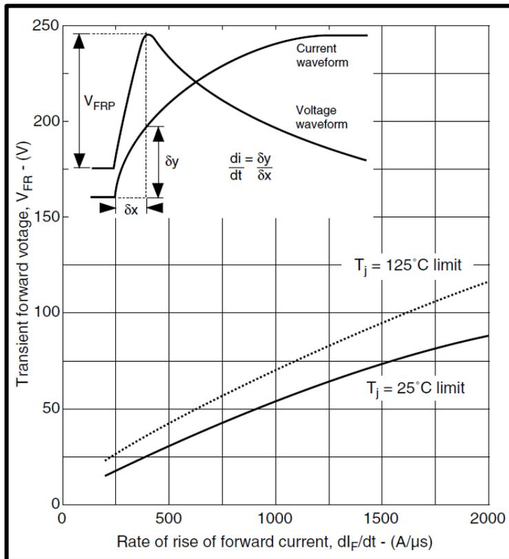
Fig.7 Transient forward voltage
