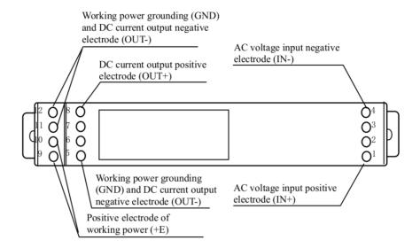
\*The undefined terminals in the diagram can't be used.
