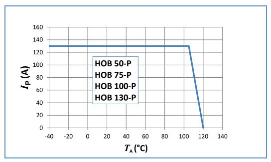
Important notice: whatever the usage and/or application, the transducer jumper temperature shall not go above the maximum rating of 120 °C as stated in page 3 of this datasheet.
