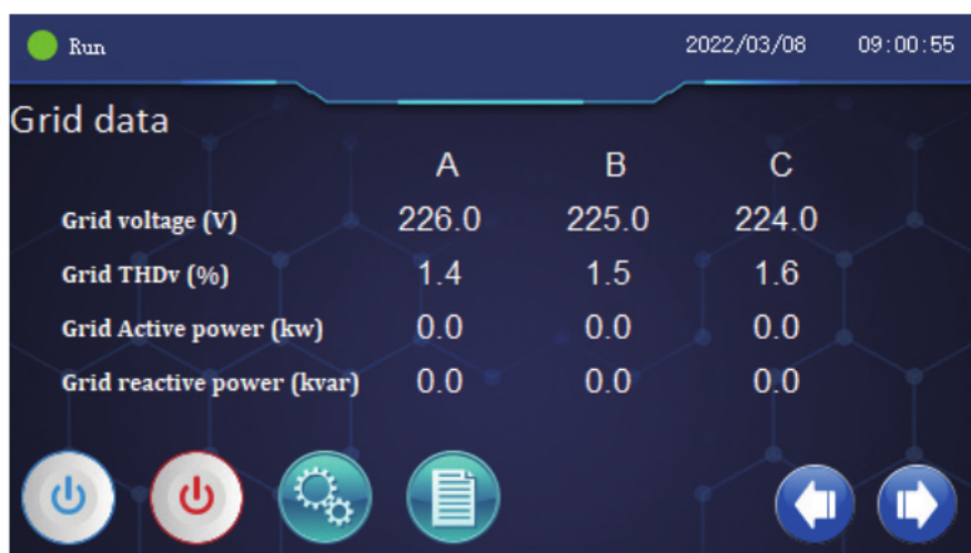
Figure 2 Touch screen main interface
