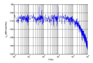
Figure 13: Typical noise power density of V ( $R_{\rm M}$ ) with  $R_{\rm M}$  = 50  $\Omega$
