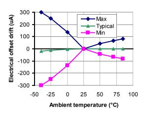
Figure 3: Electrical offset thermal drift
