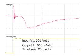
Figure 11: Typical common mode perturbation (1200 V step with 6 kV/ $\mu$ s  $R_{\rm M}$  = 100  $\Omega$ )
