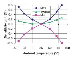
Figure 5: Sensitivity thermal drift
