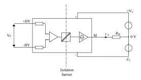
Figure 16: standard characterization schematics for current output transducers ( $R_{\rm M}$  = 50  $\Omega$  unless otherwise noted)
