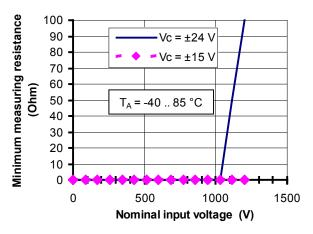
Figure 2: Minimum measuring resistance; For  $\mathbf{T}_{A}$  under 80°C, the minimum measuring resistance is 0  $\Omega$  whatever  $\mathbf{V}_{C}$
