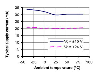
Figure 8: Supply current function of temperature
