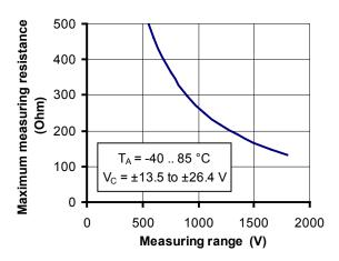
Figure 1: Maximum measuring resistance
