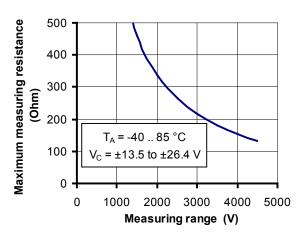
Figure 1: Maximum measuring resistance
