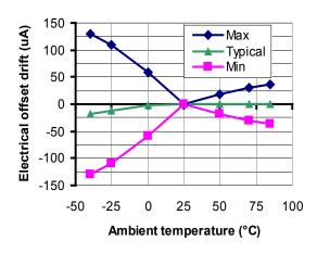
Figure 3: Electrical offset thermal drift
