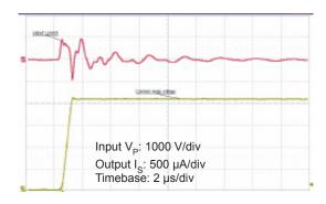
Figure 12: Detail of typical common mode perturbation (2800 V step with 6 kV/ $\mu$ s,  $R_{\rm M}$  = 100  $\Omega$ )
