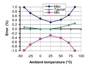
Figure 4: Overall accuracy in temperature
