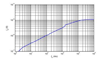
Figure 14: Typical total output current noise (rms) with  $\mathbf{R}_{\mathrm{M}}$  = 50  $\Omega$  (fc is upper cut off frequency of bandpass, low cut off frequency is 1 Hz)
