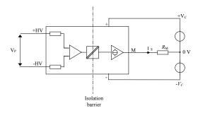
standard characterization schematics for current output transducers ( $R_{\rm M}$  = 50  $\Omega$  unless otherwise
