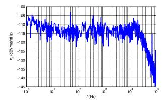
Figure 13: Typical noise power density of V ( $\mathbf{R}_{\mathrm{M}}$ ) with  $\mathbf{R}_{\mathrm{M}}$  = 50  $\Omega$
