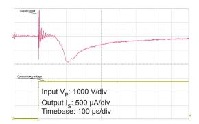
Figure 11: Typical common mode perturbation (2800 V step with 6 kV/ $\mu$ s  $R_{\rm M}$  = 100  $\Omega$ )
