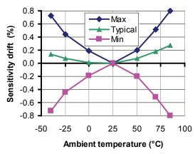
Figure 5: Sensitivity thermal drift
