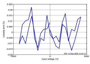
Figure 15: Typical linearity error
