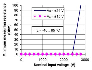
Figure 2: Minimum measuring resistance; For  $\mathbf{T}_{A}$  under 80°C, the minimum measuring resistance is 0  $\Omega$  whatever  $\mathbf{V}_{C}$
