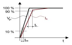
Figure 18: response time  $t_r$  and reaction time  $t_{ra}$
