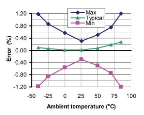
Figure 4: Overall accuracy in temperature
