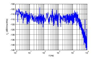
Figure 13: Typical noise power density of V ( $\mathbf{R}_{_{M}}$ ) with  $\mathbf{R}_{_{M}}$  = 50  $\Omega$
