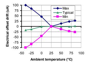
Figure 3: Electrical offset thermal drift
