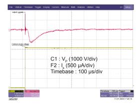
Figure 11: Typical common mode perturbation (4200 V step with 6 kV/µs,  $\mathbf{R}_{\rm M}$  = 100 Ω)
