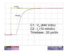
Figure 6: Typical step response (0 to 4200 V)
