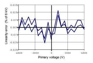
Figure 15: Typical linearity error
