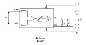
Figure 17: standard characterization schematics for voltage output transducers ( $\mathbf{R}_{_M} = 100 \text{ k}\Omega$  unless otherwise noted)
