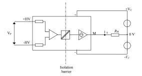
Figure 16: standard characterization schematics for current output transducers ( $\mathbf{R}_{_{M}} = 50 \ \Omega$  unless otherwise noted)
