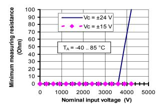
Figure 2: Minimum measuring resistance Under  $T_A = 80$ °C, the minimum measuring resistance is 0 whatever Vc
