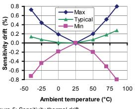
Figure 5: Sensitivity thermal drift
