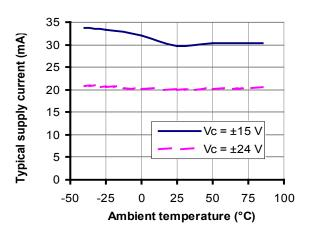
Figure 8: Supply current function of temperature
