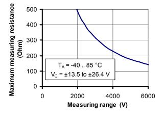
Figure 1: Maximum measuring resistance
