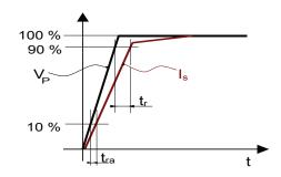
Figure 18: response time  $t_r$  and reaction time  $t_r$
