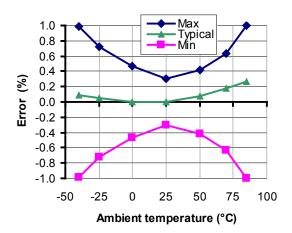
Figure 4: Overall accuracy in temperature
