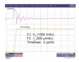
Figure 12: Detail of typical common mode perturbation (4200 V step with 6 kV/ $\mu$ s,  $R_{\rm M}$  = 100  $\Omega$  )
