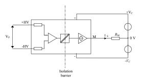
Figure 16: standard characterization schematics for current output transducers ( $R_{\rm M}$  = 50  $\Omega$  unless otherwise
