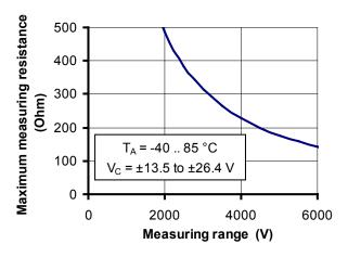
Figure 1: Maximum measuring resistance
