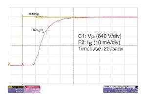
Figure 6: Typical step response (0 to 4200 V)
