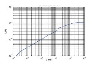
Figure 14: Typical total output current noise (rms) with  $\mathbf{R}_{_{\mathrm{M}}}$  = 50  $\Omega$  (fc is upper cut off frequency of bandpass, low cut off frequency is 1 Hz)
