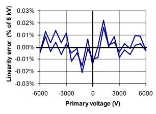
Figure 15: Typical linearity error
