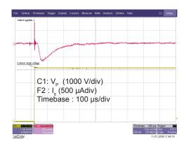
Figure 11: Typical common mode perturbation (4200 V step with 6 kV/ $\mu$ s,  $R_{\rm M}$  = 100  $\Omega$ )
