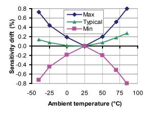
Figure 5: Sensitivity thermal drift
