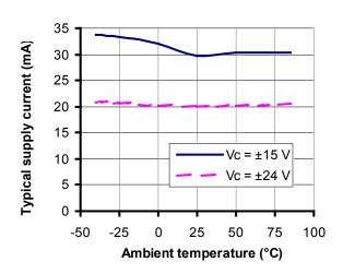
Figure 8: Supply current function of temperature
