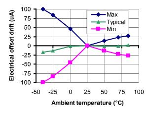
Figure 3: Electrical offset thermal drift
