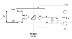
Figure 17: standard characterization schematics for voltage output transducers ( $R_{\rm M}$  = 100 k $\Omega$  unless other -wise noted)
