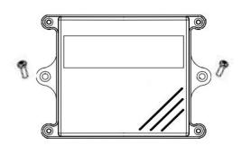
The installation port is located on both sides of the device, the diameter of the installation hole is less than 4mm, and it can be installed to the position you want to install with self-tapping screws.
