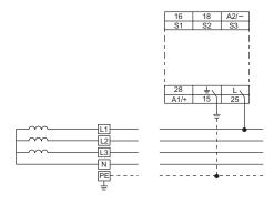
Note :- Connection of measuring input 'L' to any of the conductors
