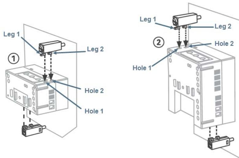
**Figure 14: Mounting the meter with the clamps**
