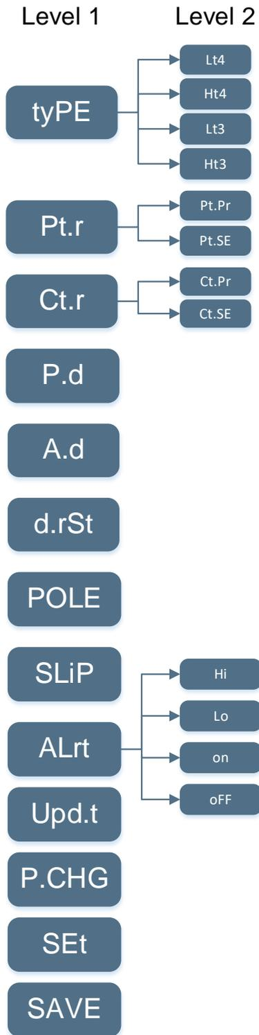
Figure 9: Menu sequence in set up mode for LED meter range
