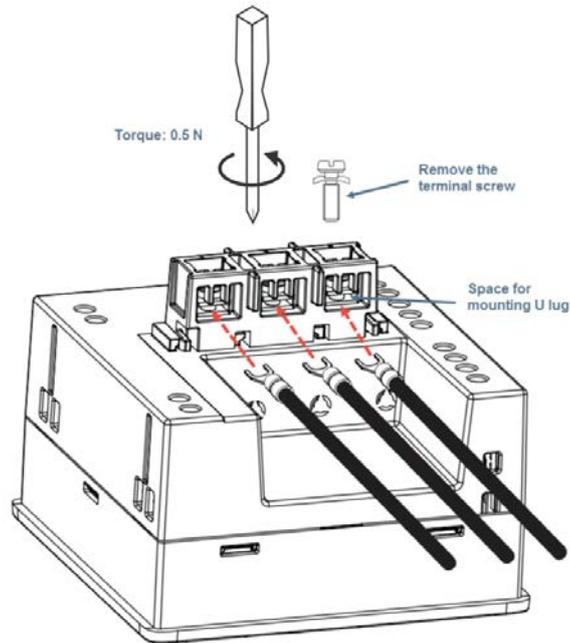
**Figure 17: U-lug wire fitting in Parking terminal**
