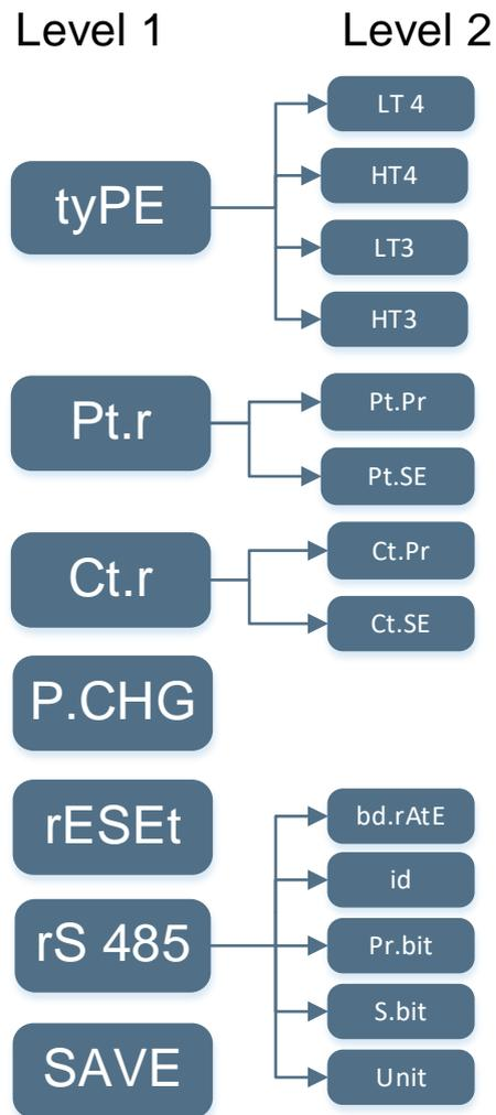
Figure 8: Menu sequence in Set-up mode (Energy meter)
