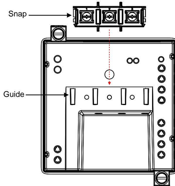
Figure 16: Parking terminal installation
