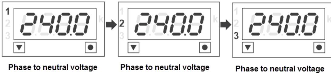
The below given cycle of displays will appear while meter is running in manual mode.
