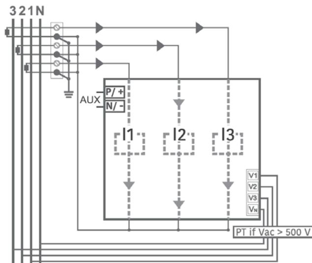
Figure 12: Making connections: 3 Phase 4 Wire connections
