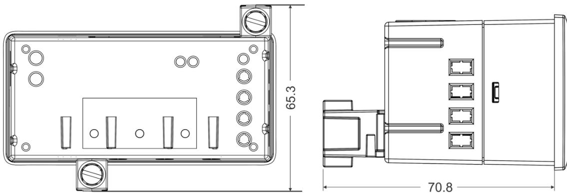
Figure 3: Meter dimensions with mounting screw and parking terminal
