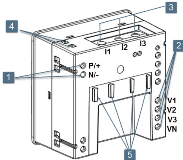
Figure 7: Rear panel details (Size: 96x96)
