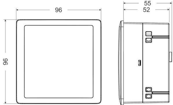
Figure 4: Meter dimensions without mounting screw and parking terminal
