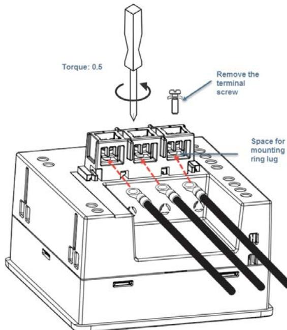
**Figure 18: Ring-lug wire fitting in Parking terminal**
