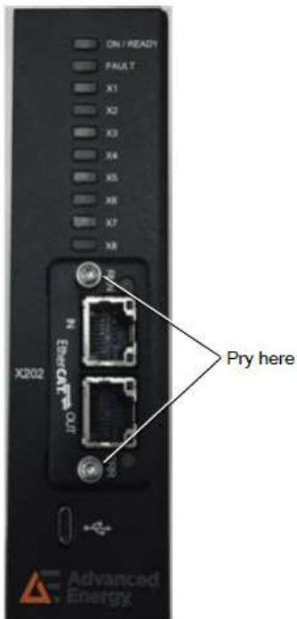
Figure 2. Anybus module removal
