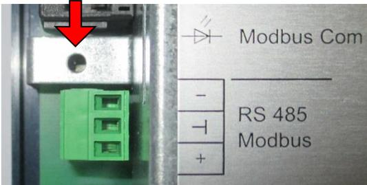
The yellow light-emitting diode at the back of the device indicates the activity of the data transmission. This only lights (flashes) when the device communicates with the master device.
