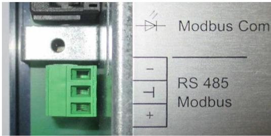
A 3-pole plug connector is provided for the connection of the Modbus interface. The symbolism in the adjacent figure illustrates the terminal assignment.
