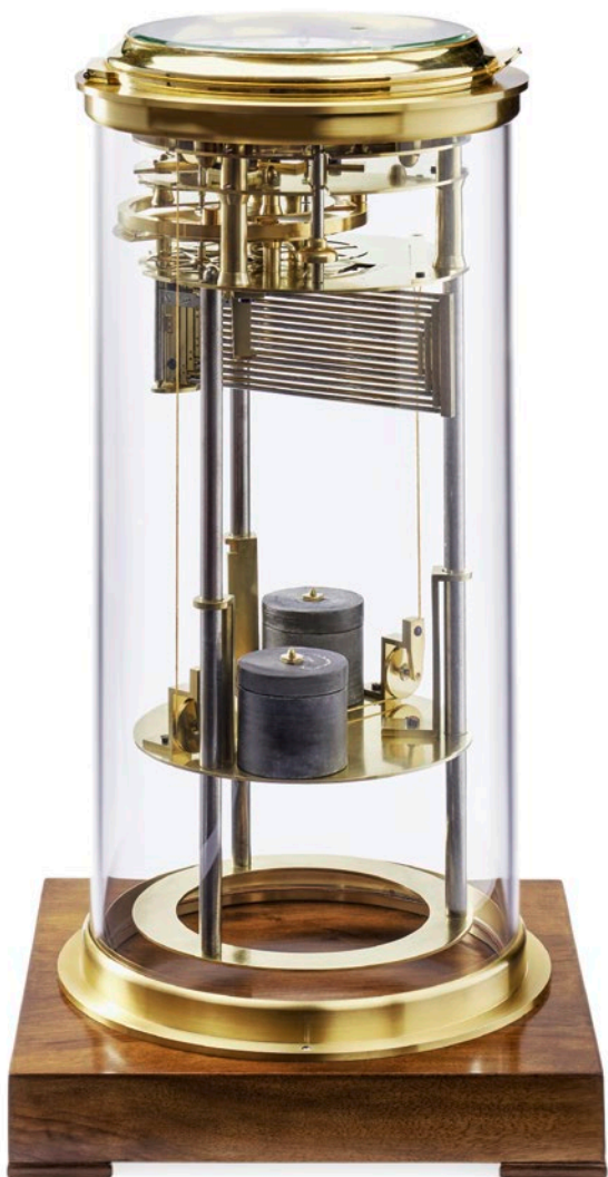
Marine Clock No. 14 by Ferdinand Berthoud, 1775. One of the eight chronometers built by the master horologist and delivered to the Spanish Navy.
