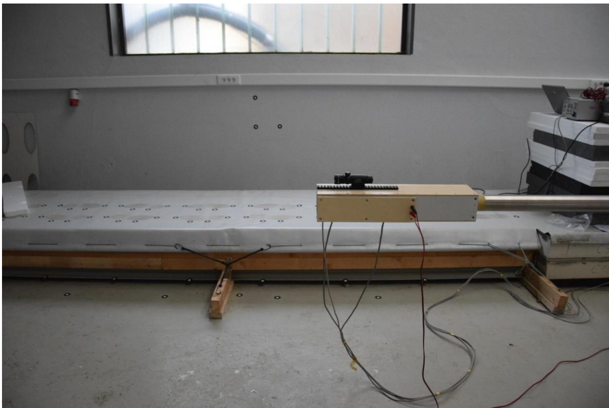
Picture 4: The velocity measurement cell on the end of the bombarding pipe.
