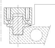
Note: Bumper stops are required. Gap approx. 2...3 mm. A special part is available with integrated bumper stops
