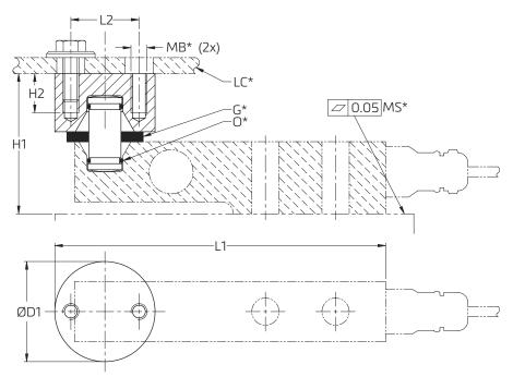
\_\_\_\_\_Detail of installation guide pin \_\_\_\_
