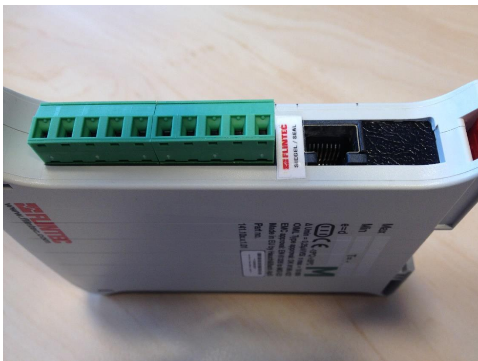
Figure 3 Sealing of DAD14x.y enclosure and calibration jumper
