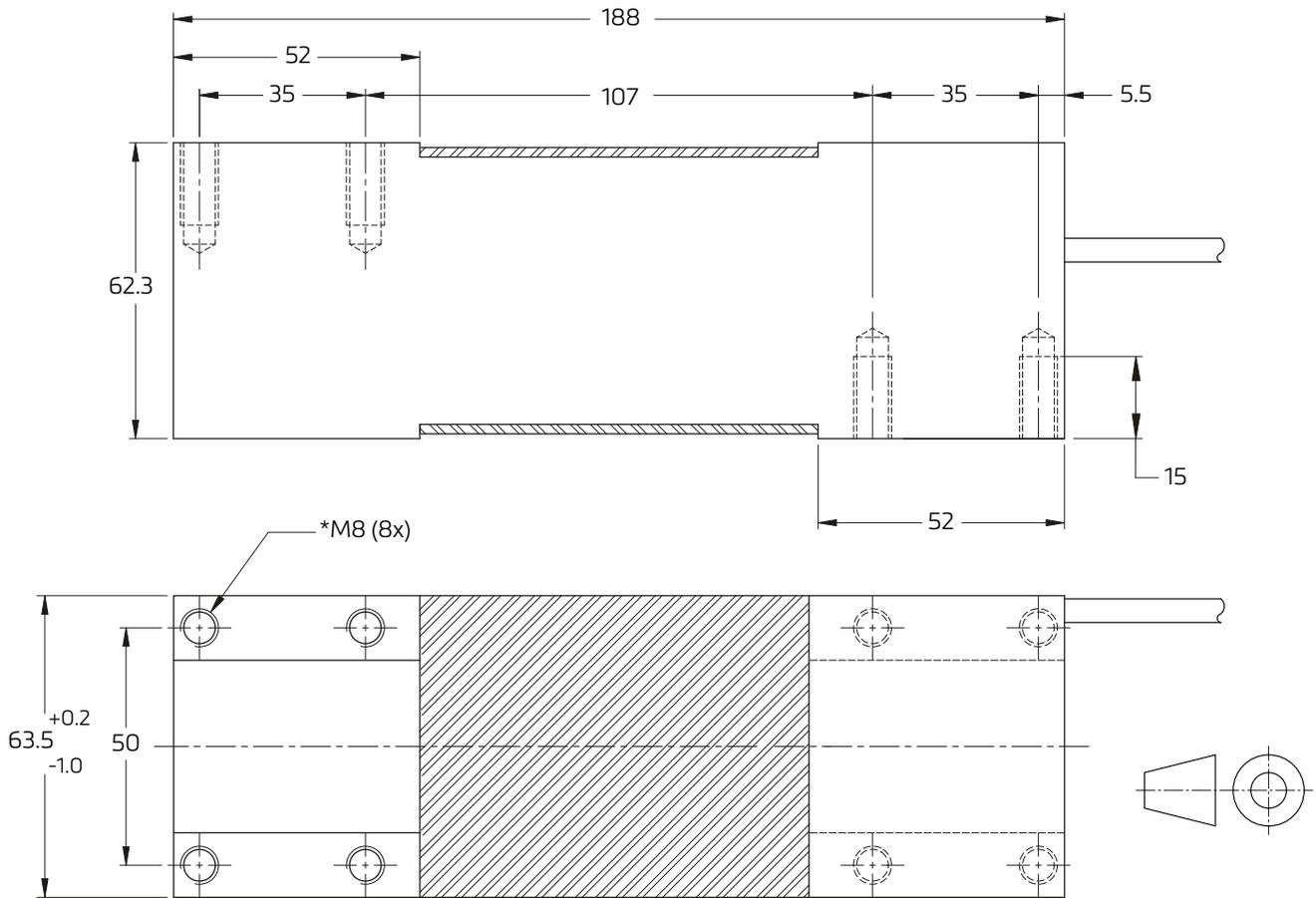
Mounting bolts M8 8.8; torque 25 Nm. Torque value assumes oiled threads.
