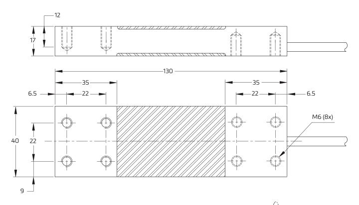
Mounting bolts M6 8.8; torque 10 Nm. Torque value assumes oiled threads.
