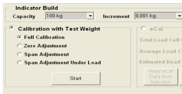
Figure 5.5 – Calibration by test weights
