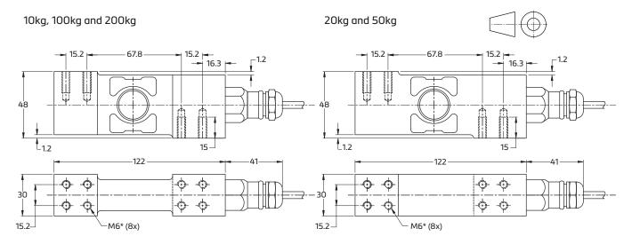
Mounting bolts M6 8.8; torque 10 Nm. Torque value assumes oiled threads.
