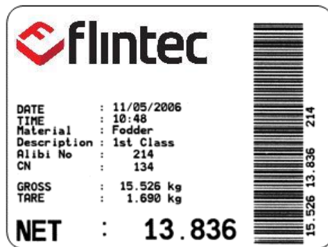
Figure 13.1- Sample of the label printout of FT-112 which is designed in EPL format.
