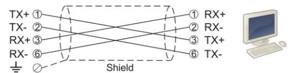
Figure 5.16 - PC connection with cross cable
