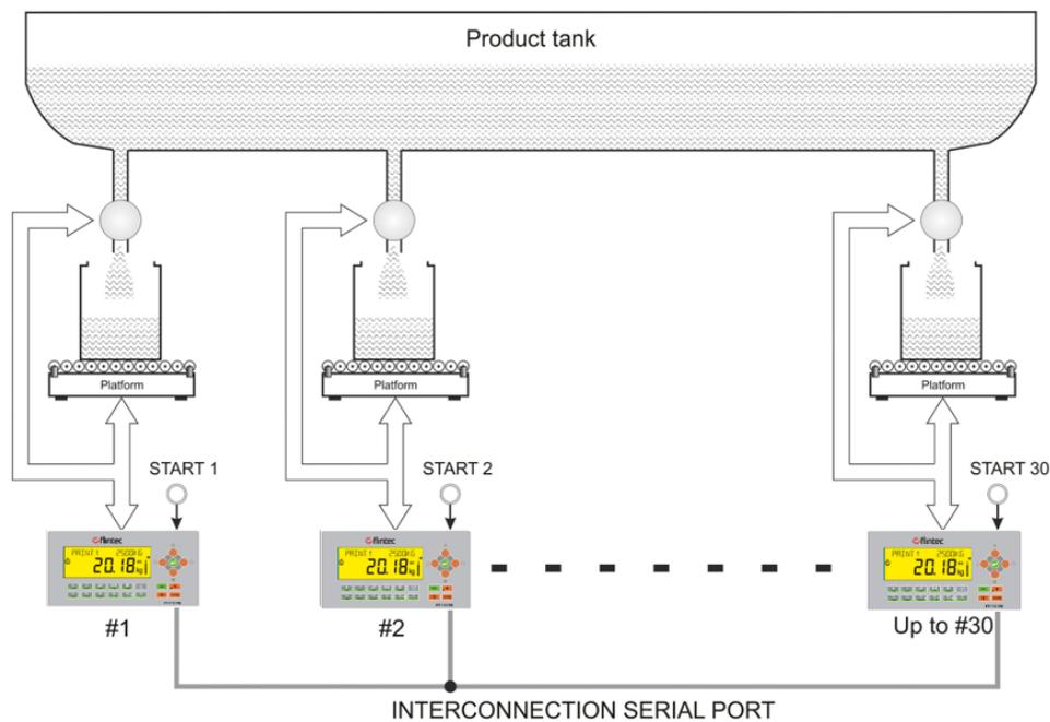
Figure 8.2 – Master slave operation at rotating filling machine
