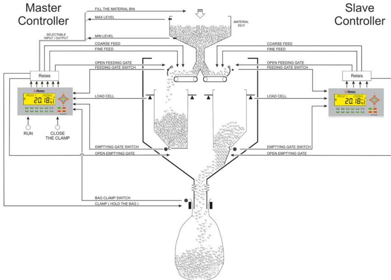
Figure 7.14 - Bagging machine with double weighing scale
