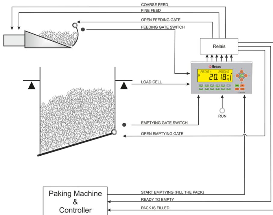
Figure 7.7 - Weighing scale control of the packing machine
