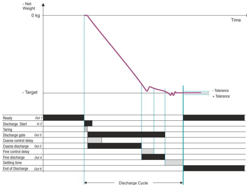
Figure 7.21 – Discharge cycle
