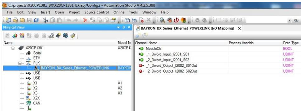
Figure 32.3 – Configuration of module properties with XDD file
