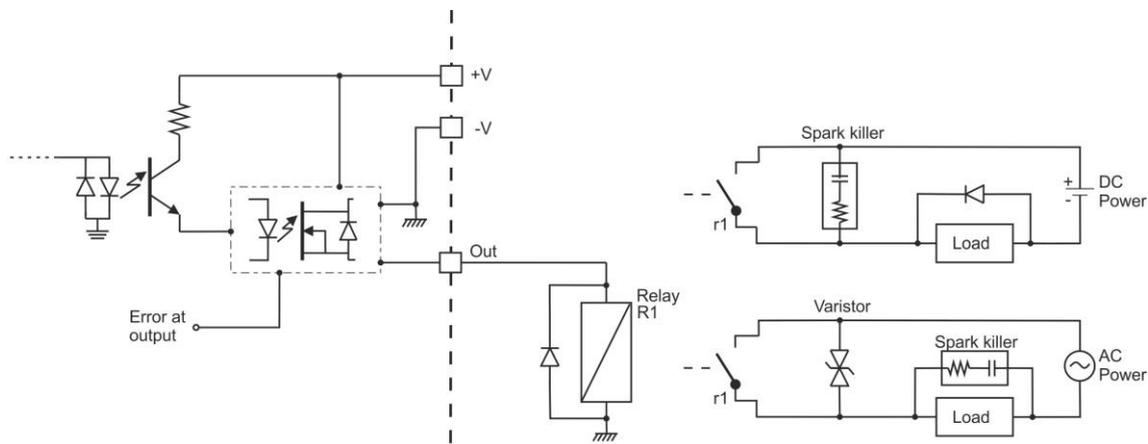
Figure 19.2 – Digital output connection diagram.
