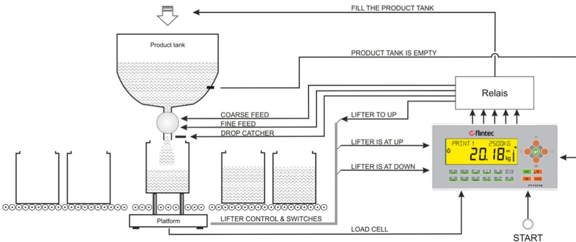
Figure 7.2 - Automatic open container filling machine with lifter
