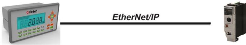
Figure 29.1 – PLC Connection
