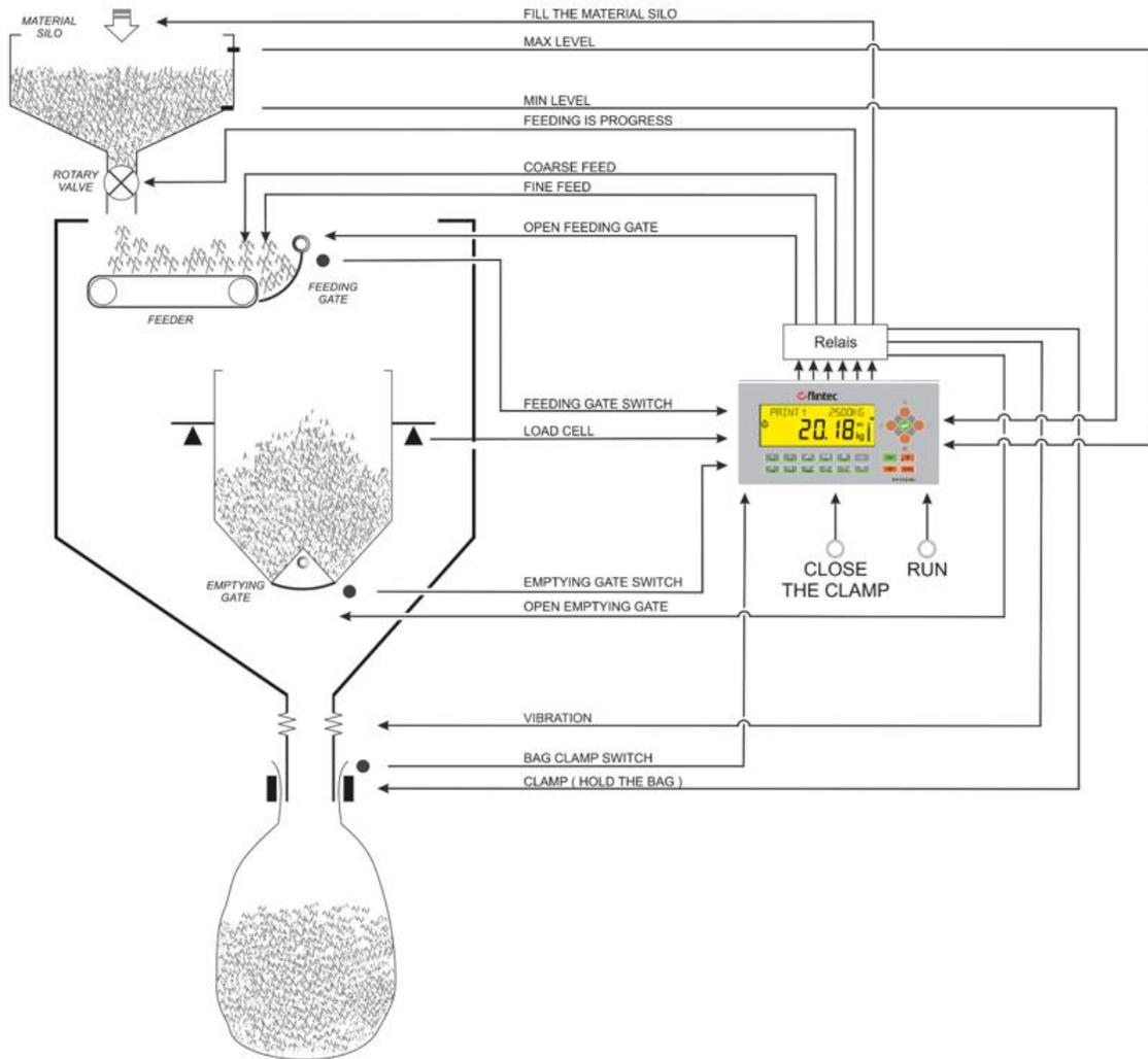
Figure 7.13 - Bagging machine with a single weighing scale
