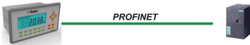
Figure 27.1 - PLC Connection
