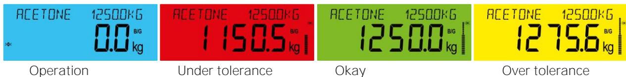
Figure 14.1 - Weight display and toolbar at filling.
