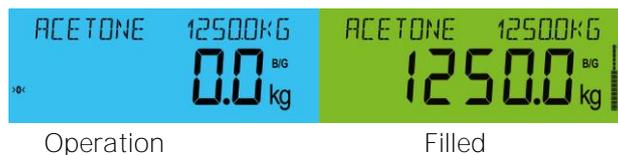
Figure 14.2 - Weight display and toolbar at filling.
