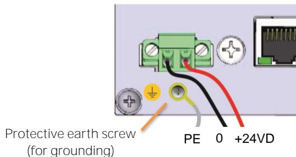
Figure 5.17 – Power source connection and grounding.
