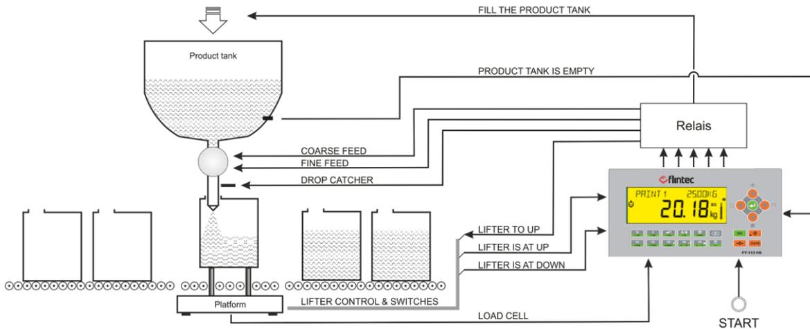
Figure 7.4 - Automatic bung hole container filling machine with container lifter
