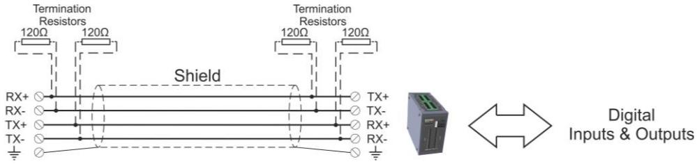
Figure 5.6 – RS422 cabling between FT-113Fill N and RIO16.
