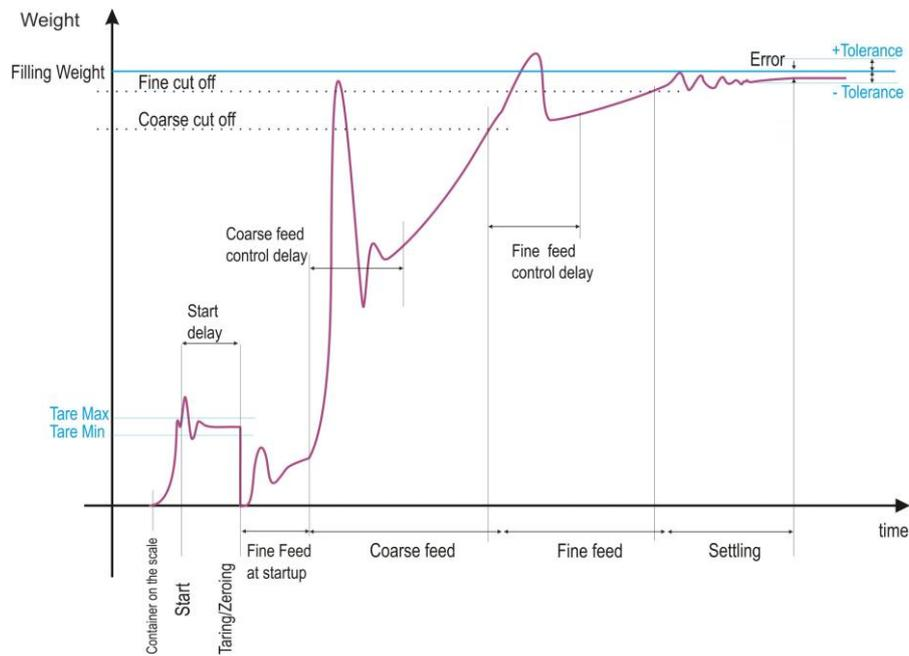
Figure 5.18 – Typical filling diagram (displayed weight vs. time)
