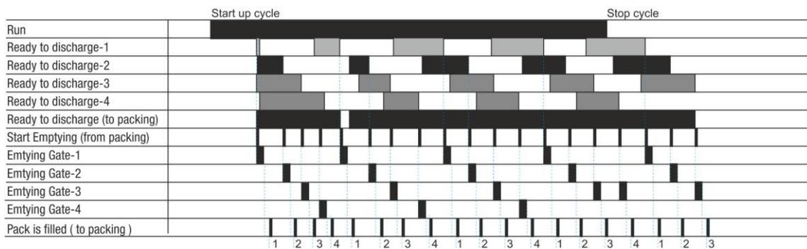
Figure 7.17 – Signalization between the weighing and packing sections of the machine.
