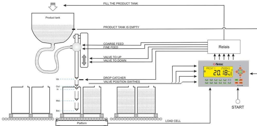
Figure 7.6 - Palette filling machine with lance control
