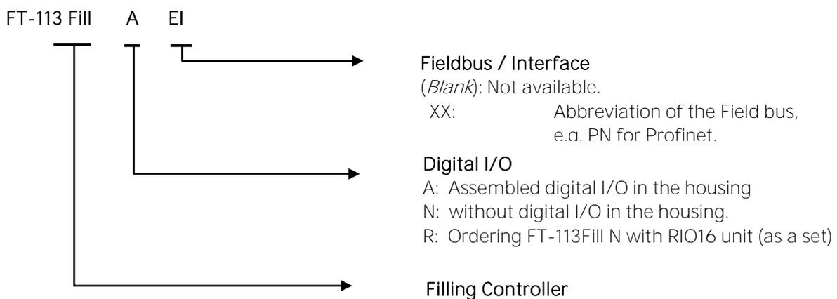
For example, the ordering code of FT-113Fill with analogue load cell input, with Profinet interface and together with the DIN rail mount digital I/O unit RIO16 is **FT-113Fill R PN**.
