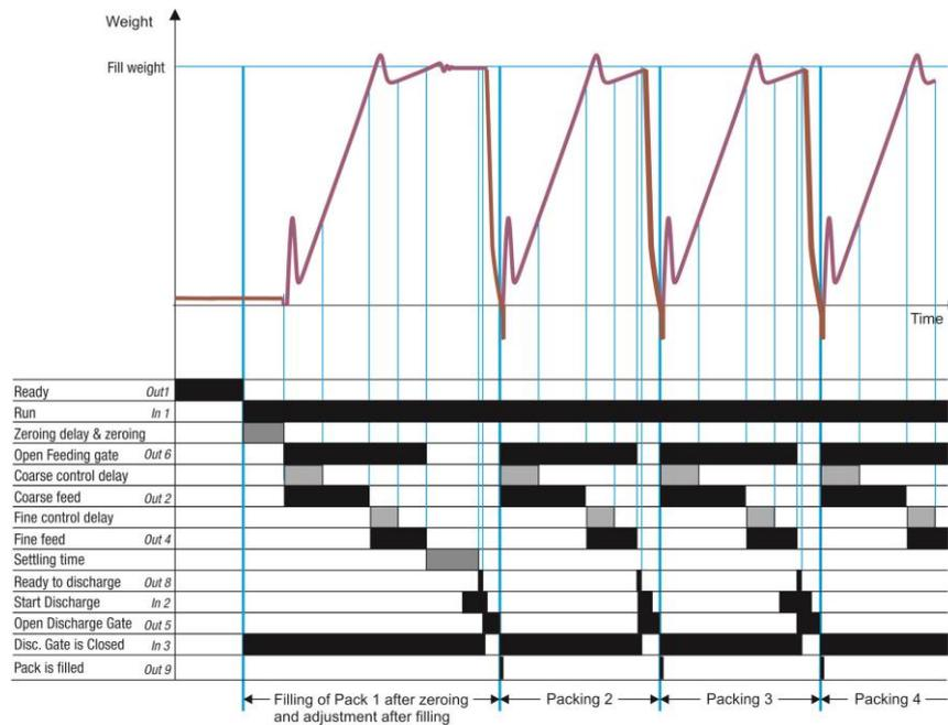
Figure 7.16 – Filling cycle for scale-1
