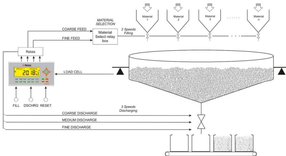
Figure 7.19 - Filling from batching scale by using very simple PLC.
