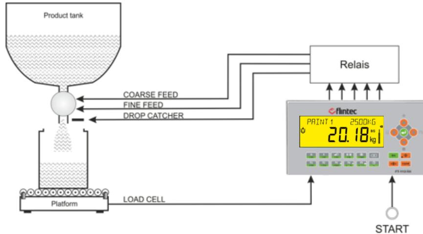
Figure 7.1 - Open container filling machine
