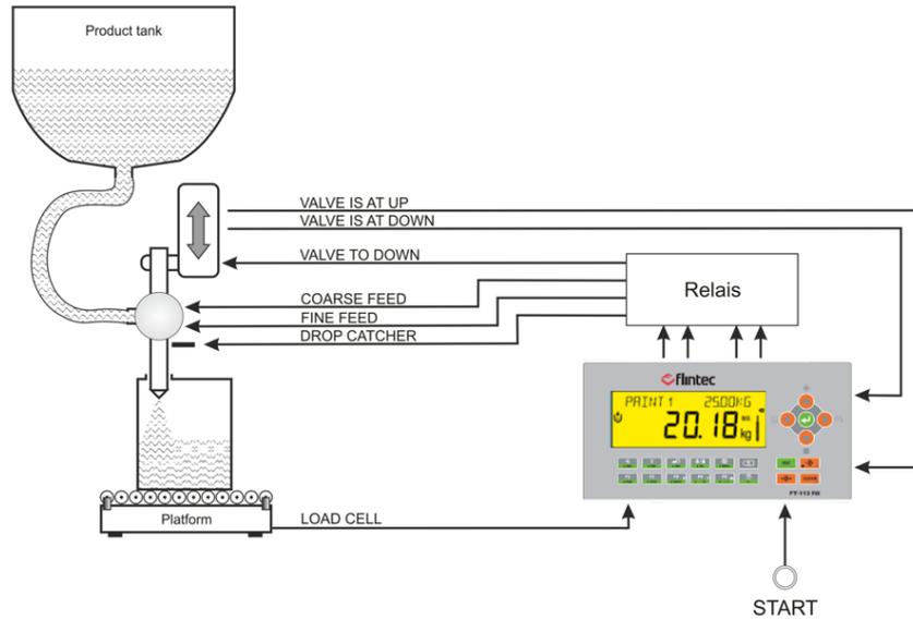
Figure 7.3 - Bung hole type container filling machine
