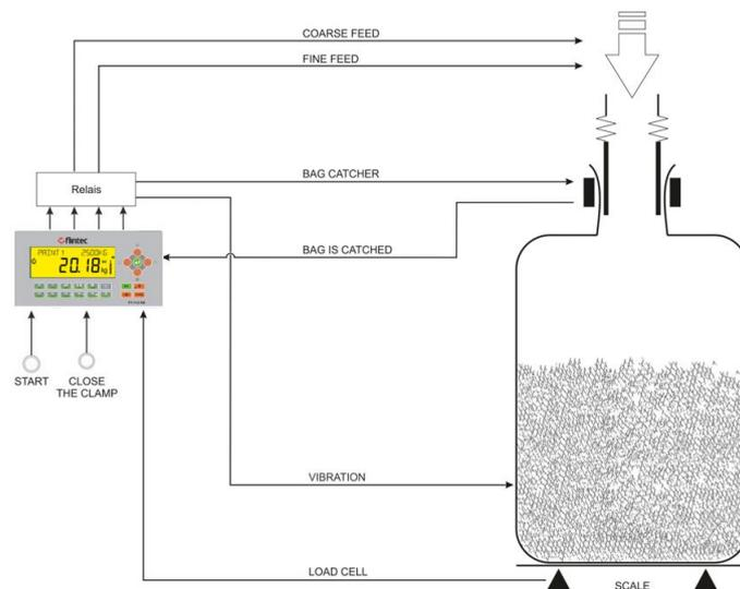
Figure 7.10 - Bag filling on the platform
