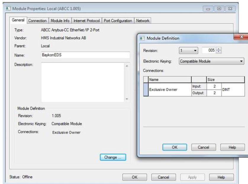
Figure 29.5 – Configuration of module properties with EDS file
