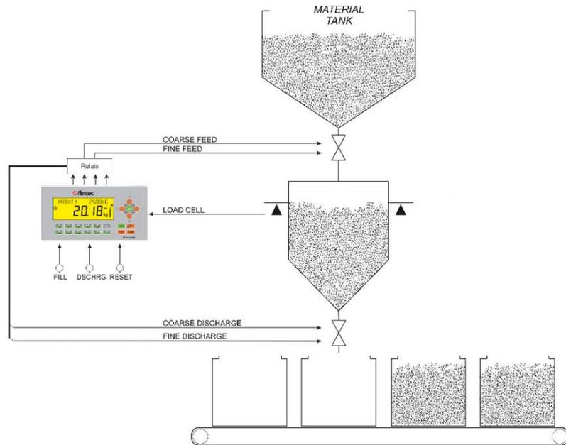
Figure 7.18 - Filling by weighing the tank or silo
