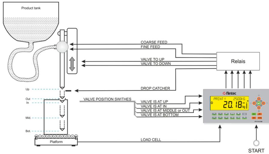
Figure 7.5 – Container filling machine with 4 position lance control
