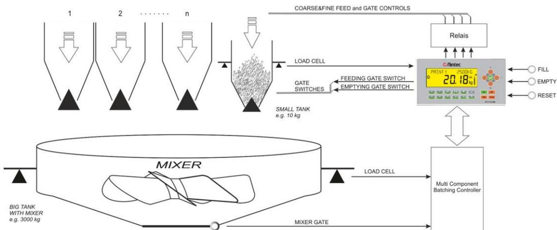
Figure 7.9 - Single material weighing at batching system
