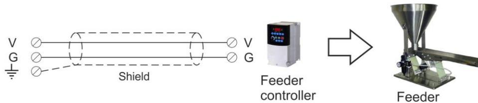
Figure 5.9 Voltage output connections
