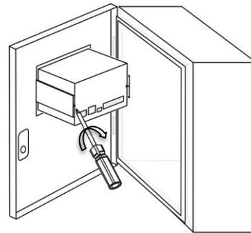
Use 2 pcs M4 screws to mount the instrument to the panel after alignment it.
