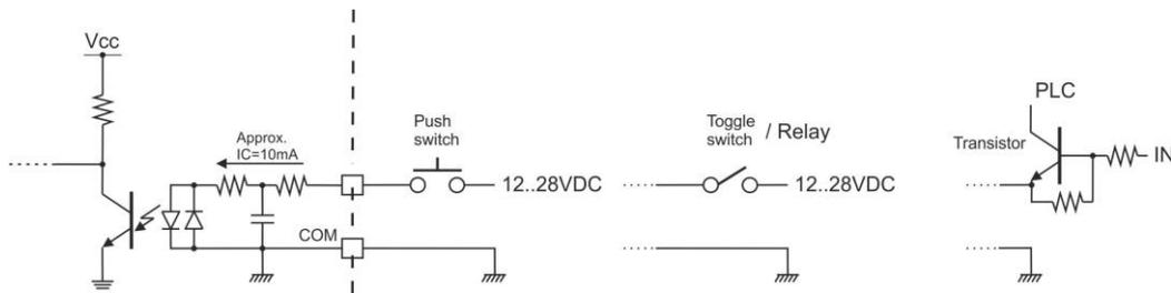
Figure 5.7 – Digital input connection diagram
