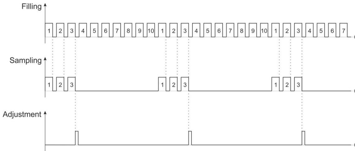
Figure 8.1 - Preact adjustment with sampling
