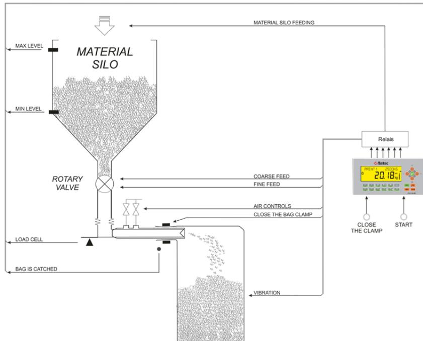
Figure 7.12 – Valve mount type bag filling machine
