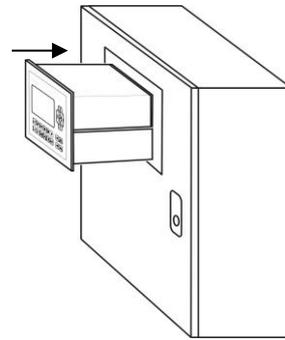
Insert the instrument into space after placing the waterproof sealing rubber behind the panel of FT-113 weighing instrument.
