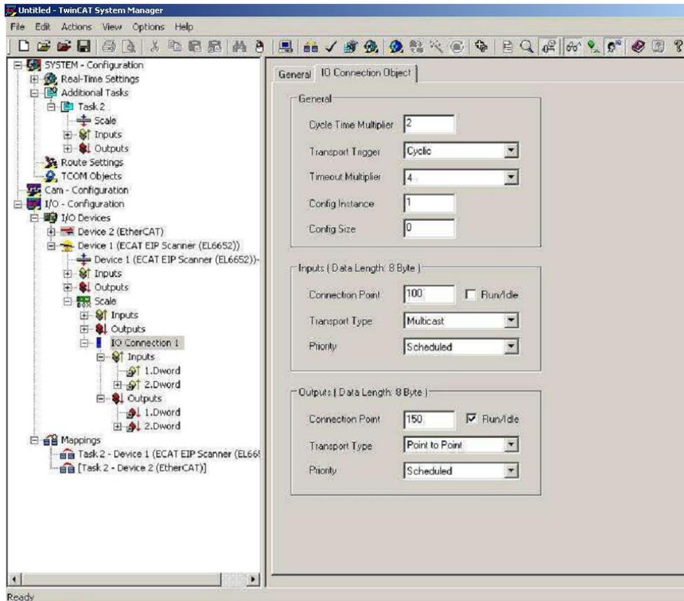
Figure 29.4 – Configuration of module properties without EDS file
