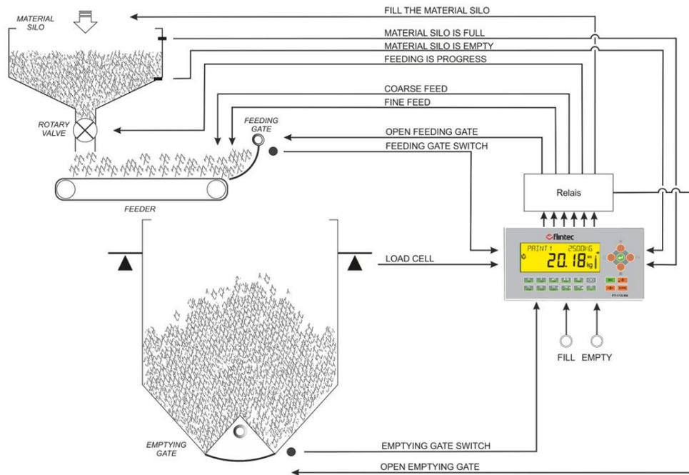
Figure 7.8 - Weighing hopper control of the Bagging machine
