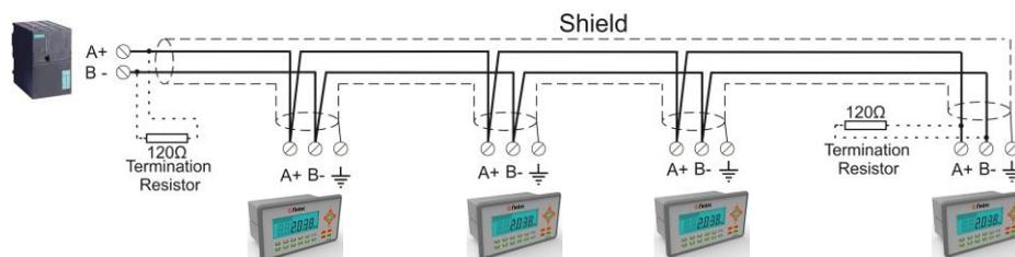
Figure 5.14 – Multi instrument connection with PLC
