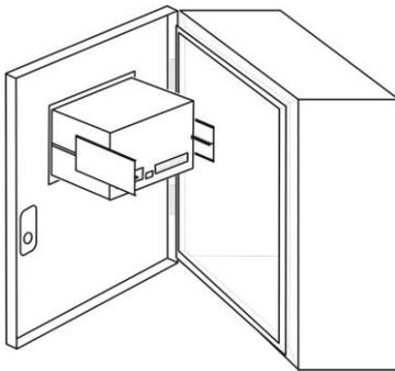
Place holder parts of the instrument to the both side of the instrument.
