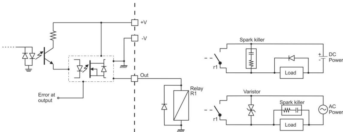
Figure 5.8 – Digital output connection diagram
