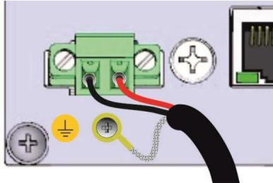
Figure 5.2– The shield connection to the protective earth.
