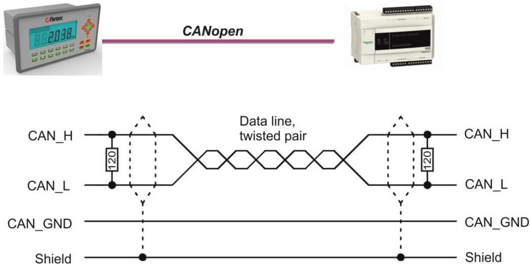
Figure 28.1 - PLC Connection
