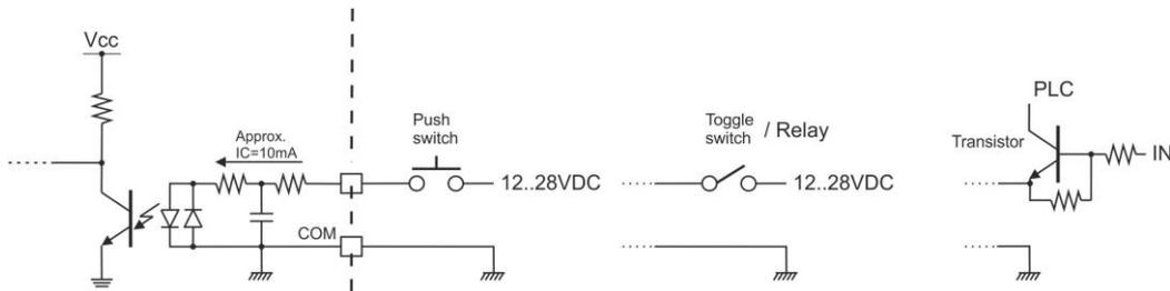
Figure 19.1 – Digital input connection diagram.
