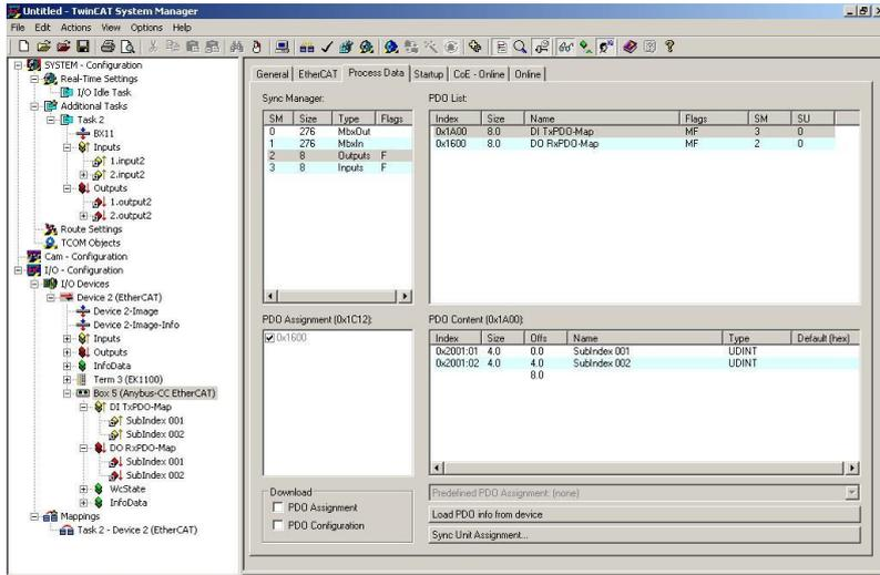
Figure 30.3 – Configuration of module properties for Beckhoff
