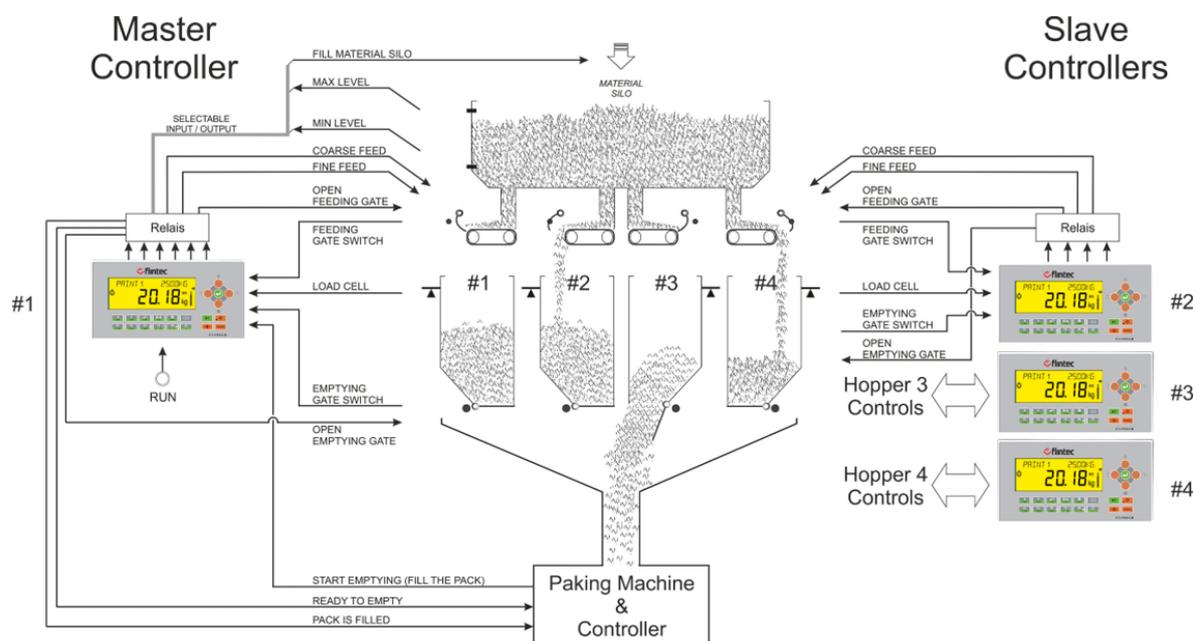
Figure 7.15 - Packing machine with four weighing scale
