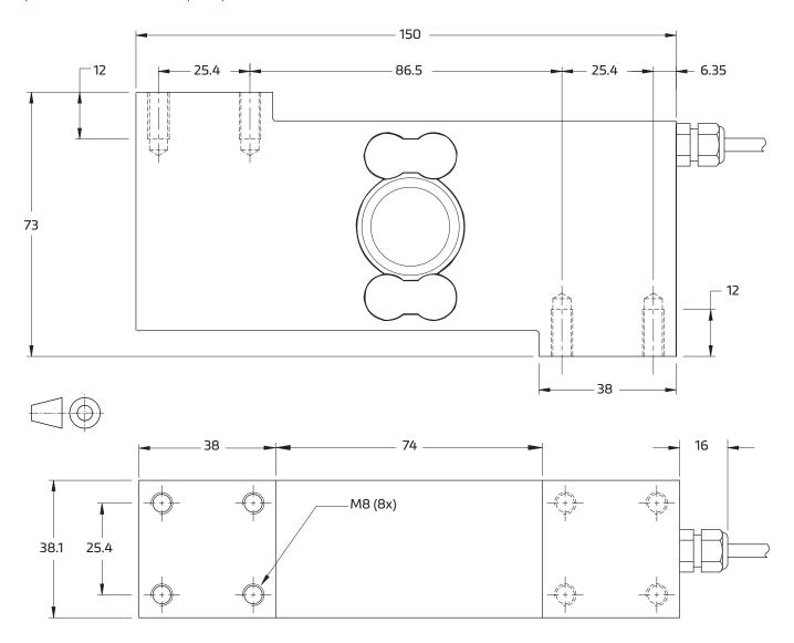
Mounting bolts M8 8.8; torque 25 Nm. Torque value assumes oiled threads.
