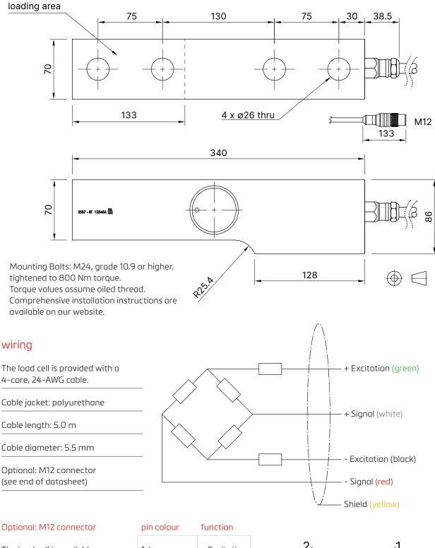
The load cell is available with an M12 connector for quick and secure installation in compatible systems. Pin assignments are shown to the right.
